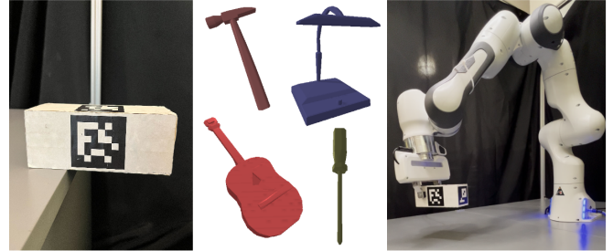
Fig. 1: Our method allows a Panda (right) to infer unobserved properties of objects based on interaction history. This allows the robot to efficiently grasp objects with non-uniform mass distributions such as weighted blocks (left) or ShapeNet objects (center).
